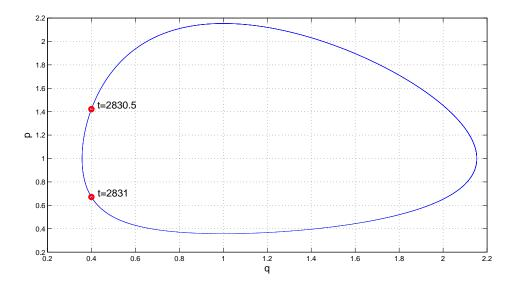
Figure 11: Trajectory in the phase plane computed by the Itoh-Abe method (33). The small circles locate the solution at the two consecutive times t=2830.5 and t=2831. The very close values of the variable q for such two points causes loss of significant digits in the subsequent branch of the trajectory.
