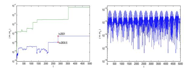
Figure 10: Left picture: absolute error of the Hamiltonian function (37) evaluated along the numerical solutions computed by the Itoh-Abe method (33) (lower curve) and formula (40)–(41) (upper curve). The jumps are symptomatic of ill-conditioning of the formulae for certain values of the solution. Right picture: the same kind of plot produced by the HBVM formula of order 4 and k=10 Gaussian abscissae ( $|H-H_0|\approx 10^{-12}$ ).
